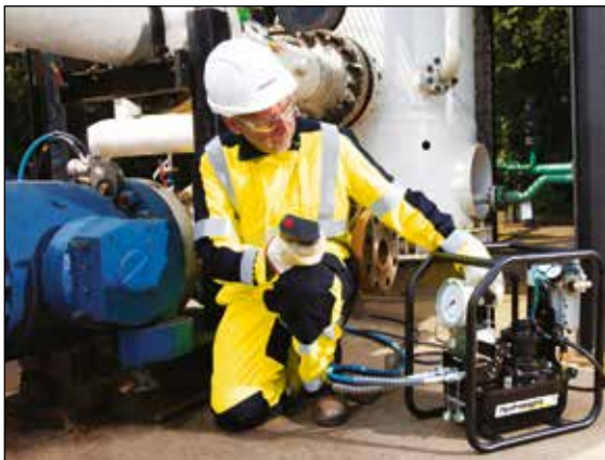
◀ Most hydraulic torque wrenches can be powered by the Enerpac ZA4T-Series torque pumps.
